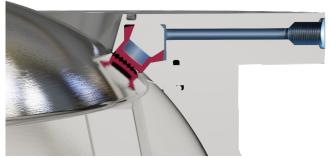
Before the ball section begins its opening rotation, the expandable air-tight seal withdraws to its safeguarded location behind the scraping ring. This design approach ensures that the seal experiences minimal shear stress, contributing to an unusually long lifespan.
