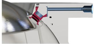
The inflatable seal is the core component of the Ball-Segment-Valve. When the seal is inflated, it closes the slight space between the segment and the scraper ring attached to the housing. The scraper ring dislodges and removes any hardened deposits on the segment before it moves past the seal. Additionally, the scraper ring stops larger particles from entering the vicinity of the inflatable seal.
