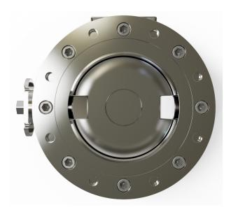
When the ball segment is closed, it shifts to the vertical CLOSED position, during which the seal is pressurized. It inflates rapidly, establishing a seal against the rounded ball segment. Once the BSV is sealed, a vessel can be swapped out as needed
